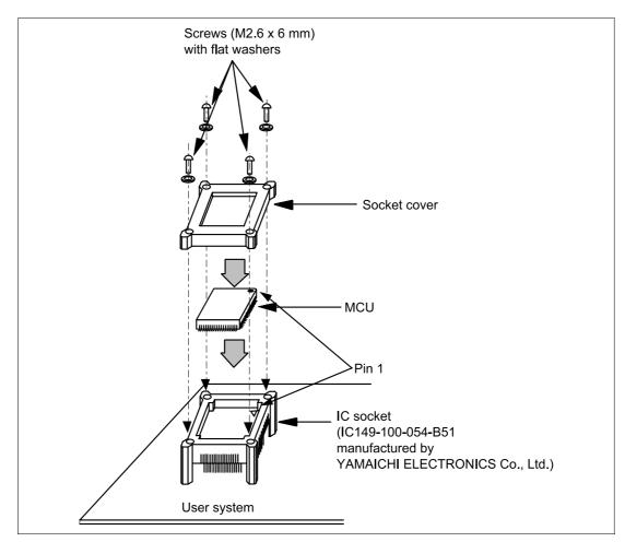
Figure 8 Installing MCU to User System
